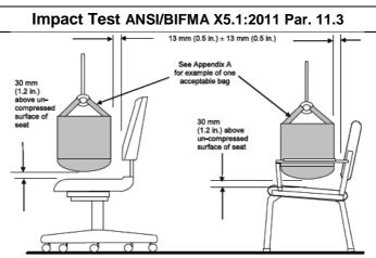
Adjustment devices have been set on the normal condition Minimum thickness of cushiony materials of seat: 0 mm Thickness of additional foam: 50 mm (IFD al 25% di 200 N  $\pm$  22 N) Distance between the bag and the backrest: 13 mm
